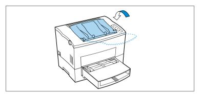
2 Press the top cover release button and open the cover.
